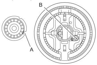
A electrode notch B ignition electrode
